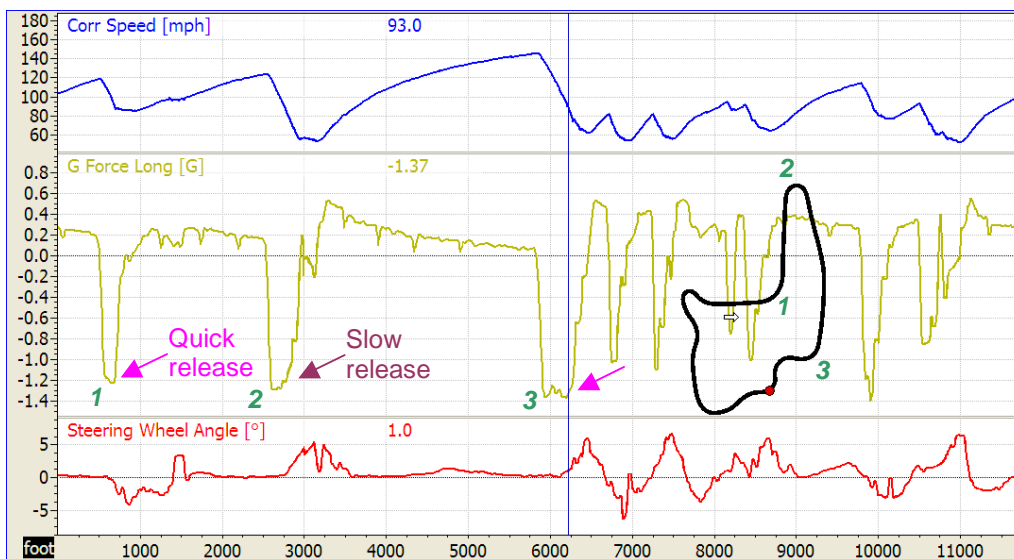
Figure 6.11 Graph for a sedan type low downforce race car at Mid-Ohio showing the braking forces from the G Force Long channel.
